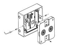
• Use only a fine tool (and no cutting tool) to puncture the center of the gasket.
